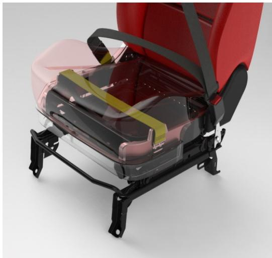
Lifebelt in an exposed concept front seat base frame
