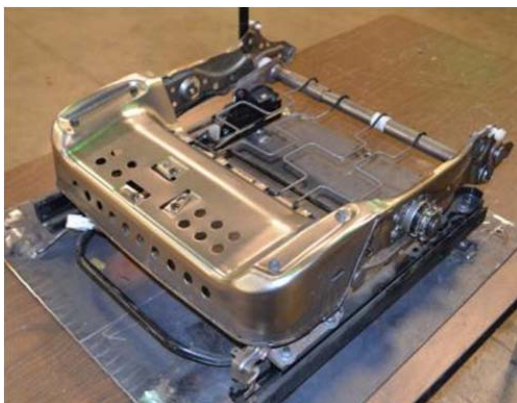
Photo 4. Model 1 structure. Sheet metal front cover over front frame tube wire seat suspension springs wrapped around rear tube.
