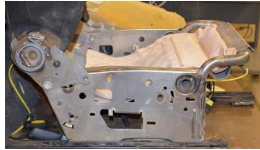
Photo 5. Model 5 seat. Sheet metal sides incorporating three cross-tubes.
