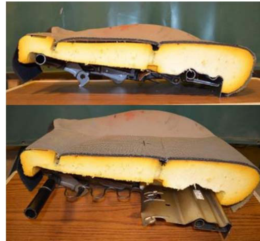
Photo 3. Cross-section of typical car seat construction. Under fabric upholstery and cushion is sheet metal cover on front of seat (to right) and a portion wire spring suspension is shown. Two side pieces are connected by a round tube in the rear and a second tube toward the front under the front cover.
