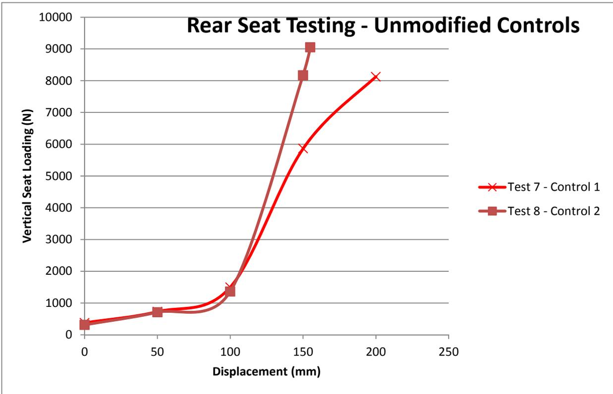
**Figure 13** Load v displacement for the standard sectioned rear passenger seat. Note that in Test 7, the rear left seat mount failed causing the seat to be depressed during the test. Testing was stopped at this point.
