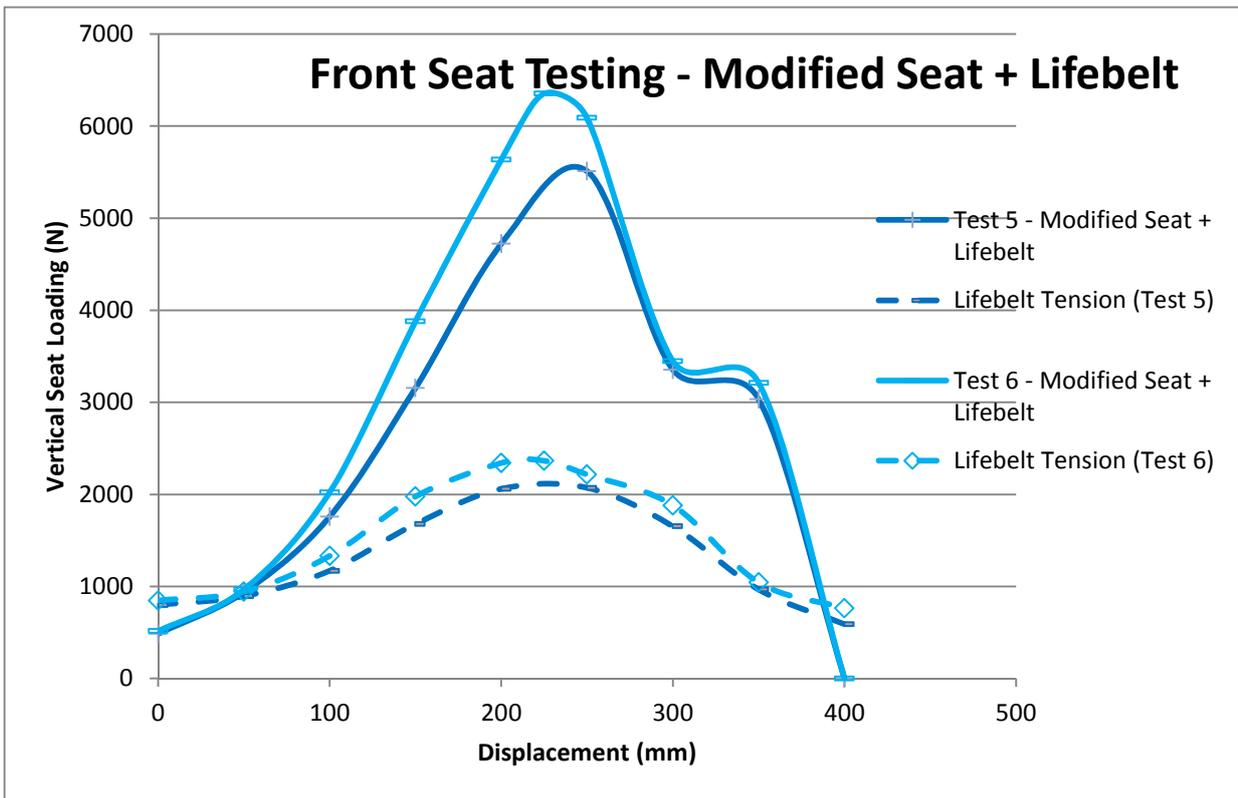
Figure 10 Load v displacement for the modified front seat fitted with the Lifebelt restraint. Note that in Tests 5 and 6, an initial tension of 800 N was applied to the Lifebelt.
