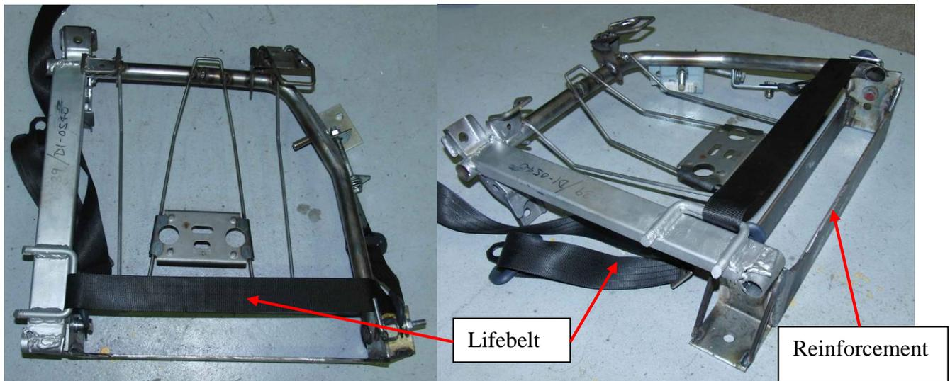
**Figure 6 Modified rear seat structure with Lifebelt position**
