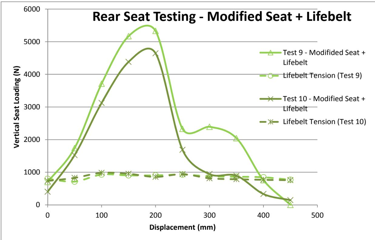
**Figure 14** Load v displacement for the modified rear passenger seat fitted with the Lifebelt restraint. Note that in Tests 9 and 10 there was inward deformation of the angle brackets anchoring the Lifebelt.
