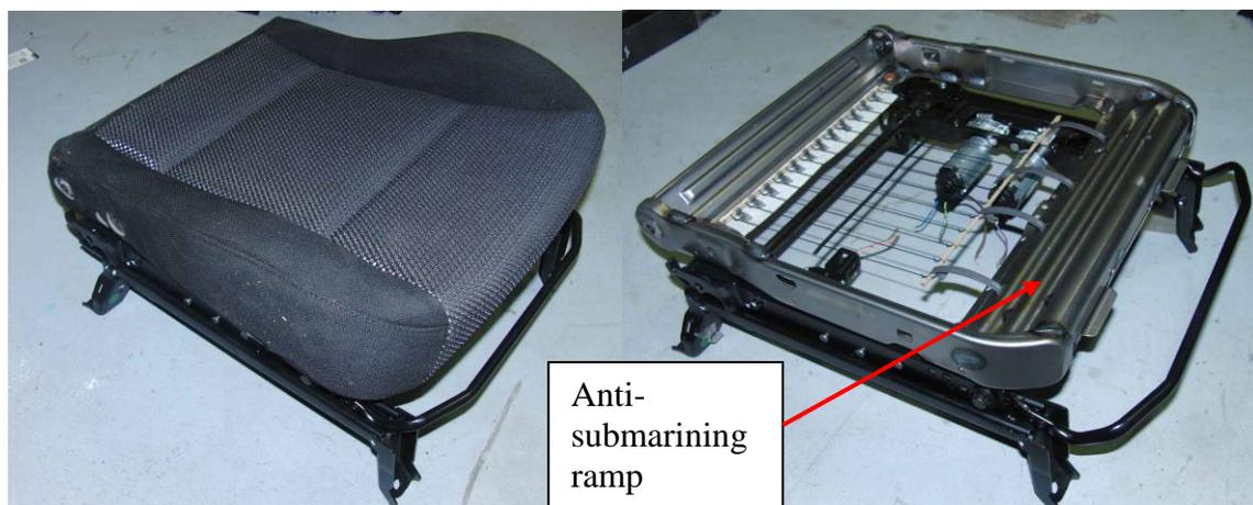
**Figure 3 Standard front seat base.**
