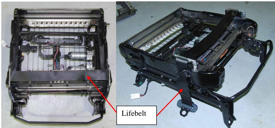
**Figure 4 The front seat base structure with Lifebelt included.**
