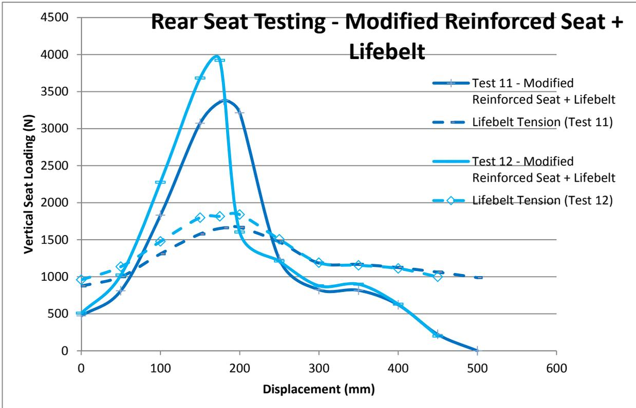
Figure 15 Load v displacement for the modified and reinforced rear passenger seat fitted with the Lifebelt restraint.
