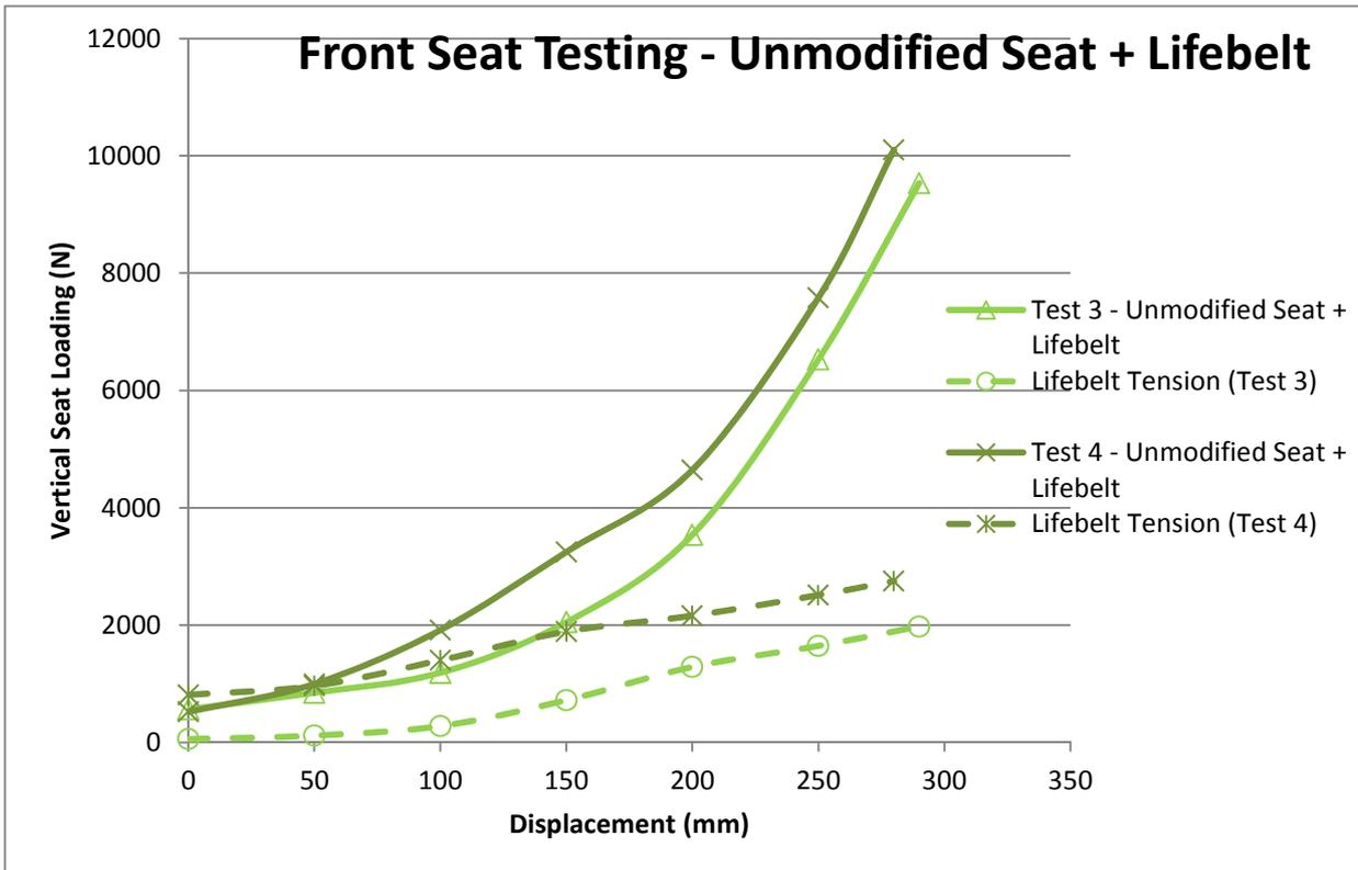
Figure 9 Load v displacement for the unmodified front seat fitted with the Lifebelt restraint. Note that the Lifebelt was not tensioned in Test 3. In Test 4, an initial tension of 800 N was applied to the Lifebelt.
