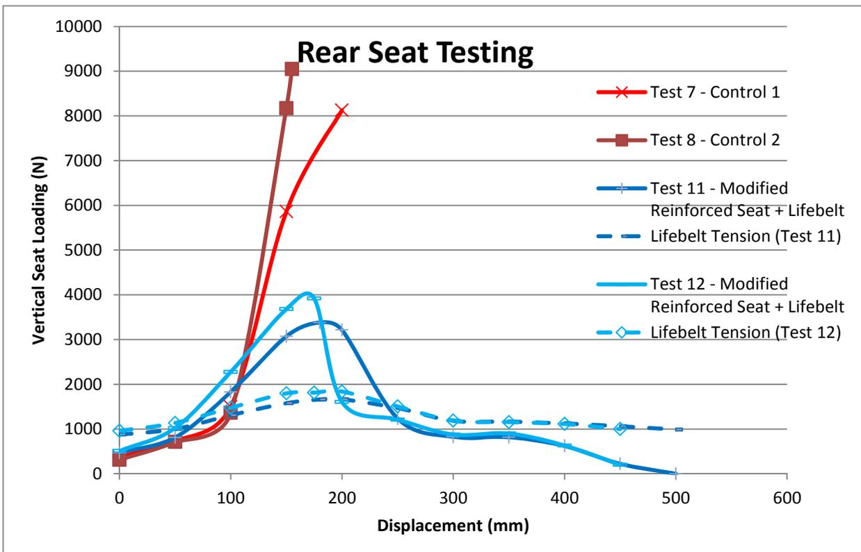
Figure 16 Load v displacement comparison between the standard rear passenger seat and the modified and reinforced rear seat fitted with the Lifebelt restraint.
