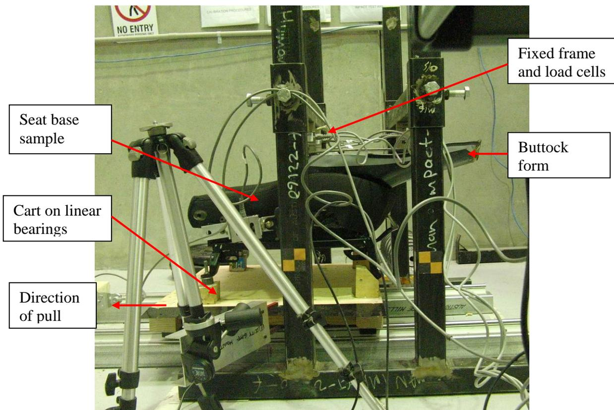
Figure 1 Static Seat Testing (SST) apparatus
