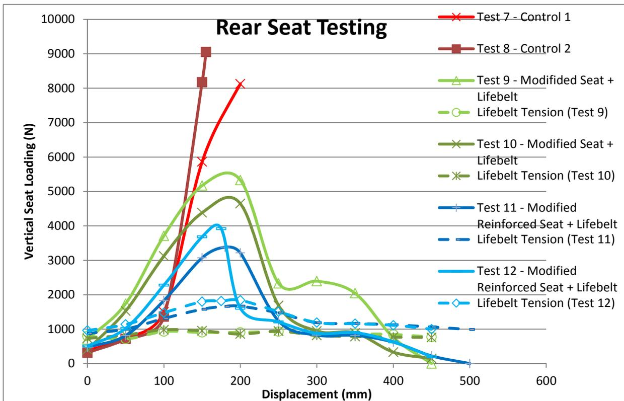
**Figure 12 Load v Displacement summary of the rear seat tests.**
