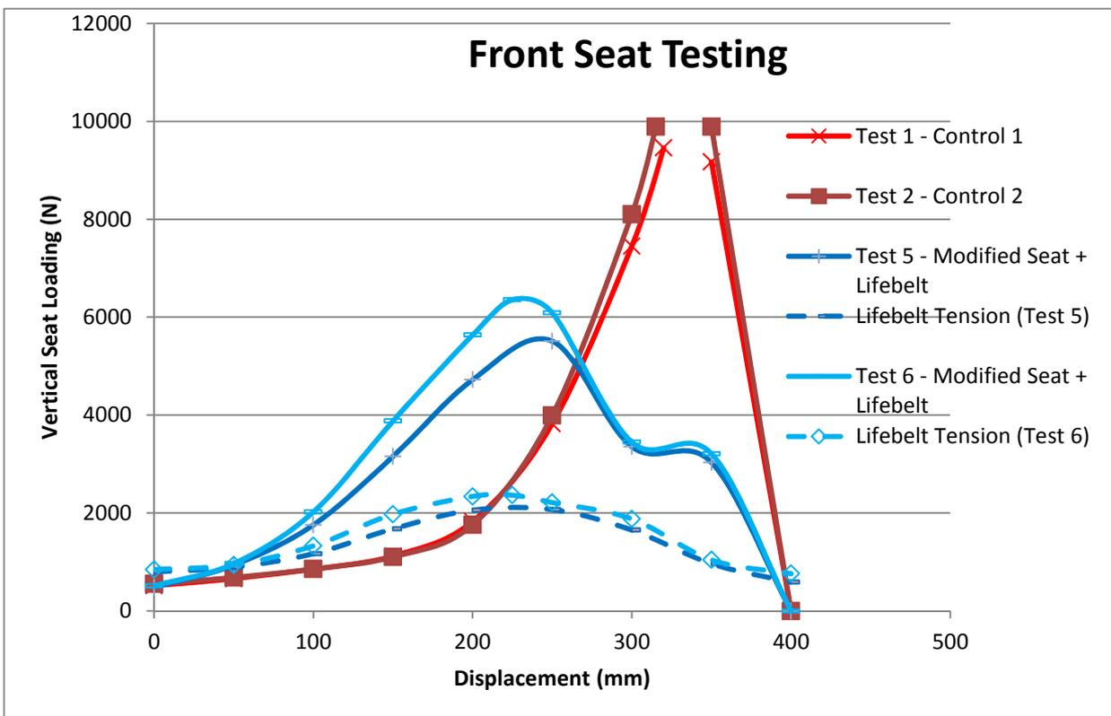
Figure 11 Load v displacement comparison between the standard unmodified front seat and the modified front seat fitted with the Lifebelt restraint.
