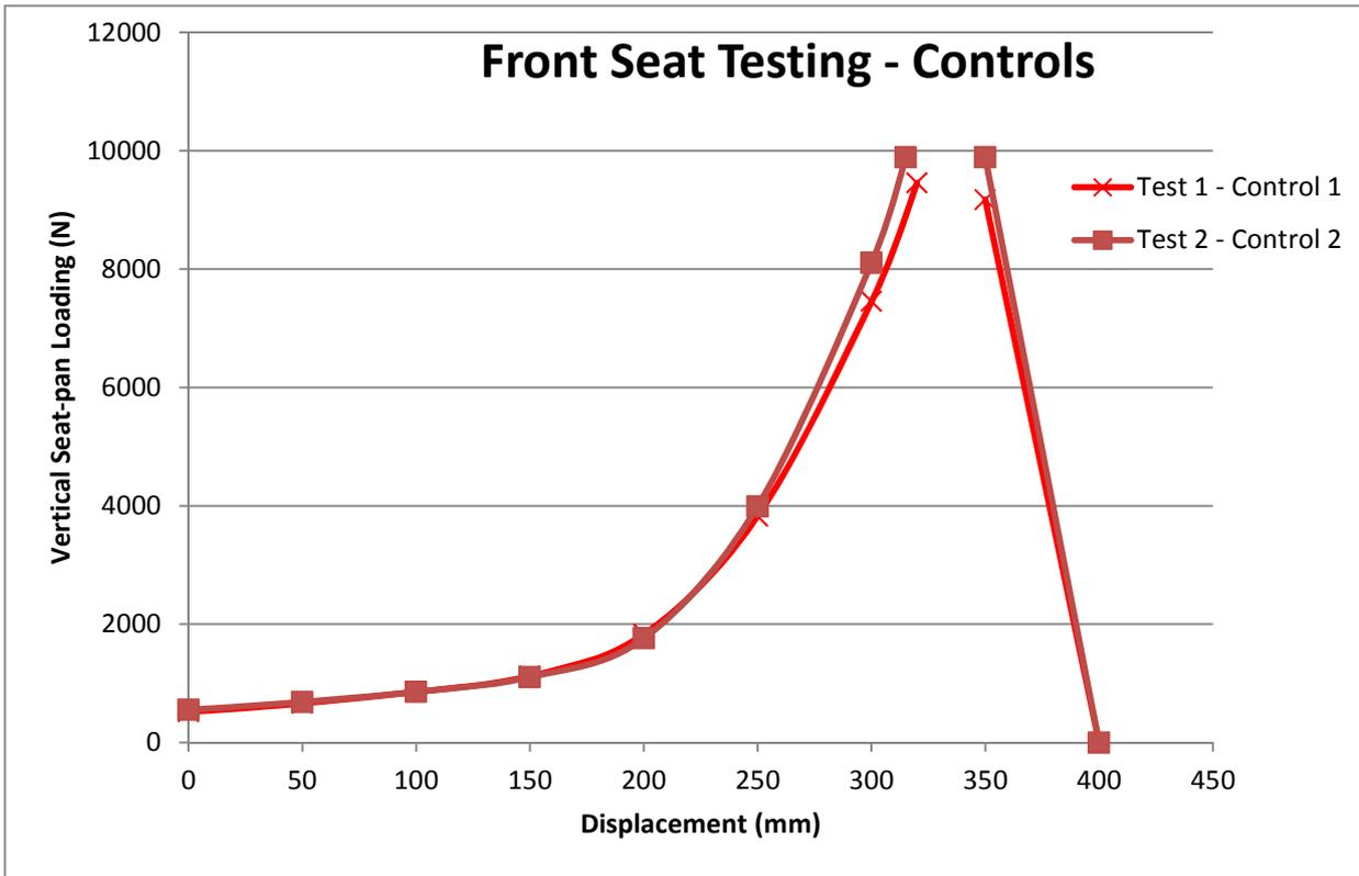
Figure 8 Load v displacement for the standard unmodified front seat.
