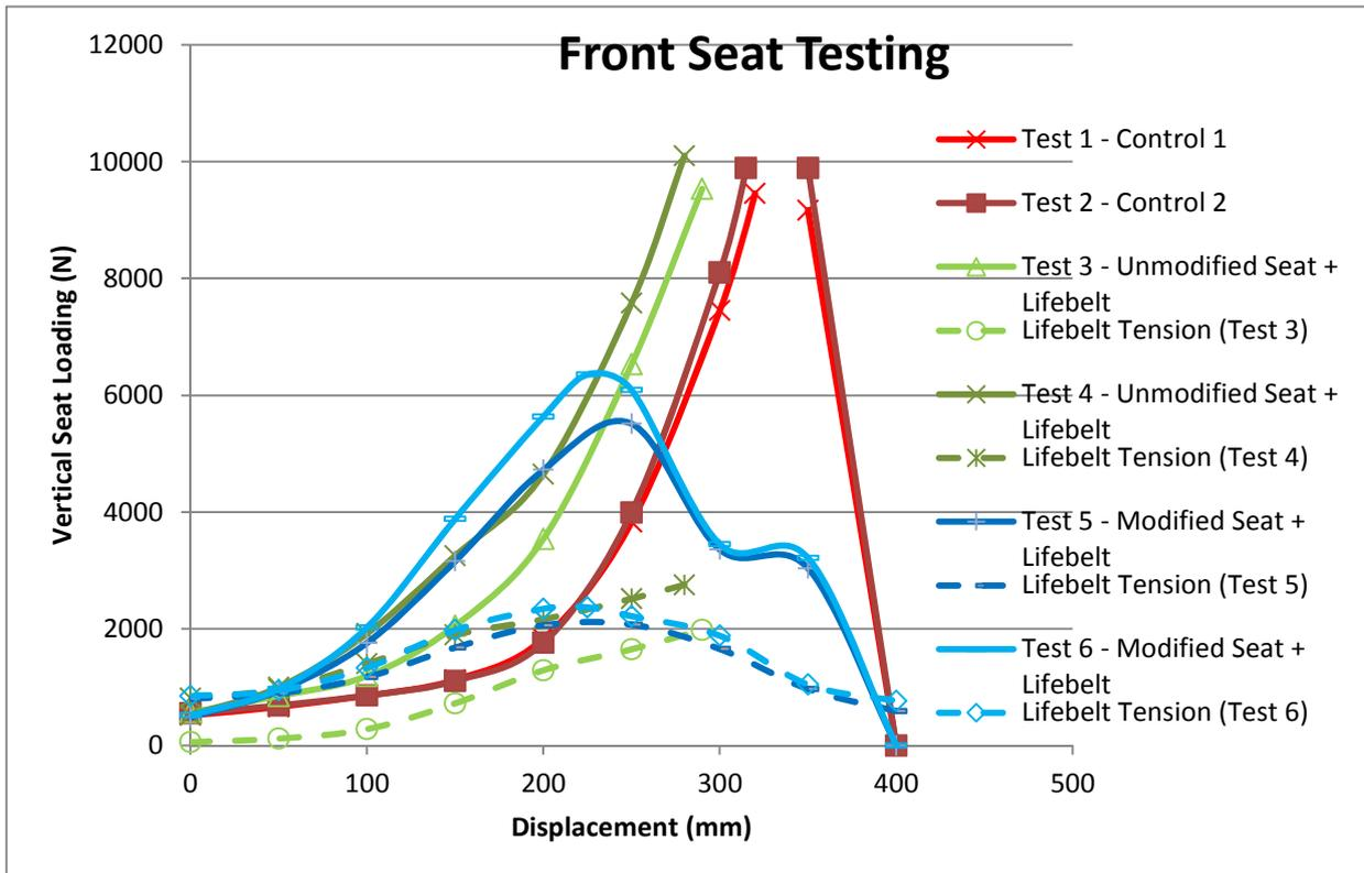
**Figure 7 Load v Displacement summary of the front seat tests.**
