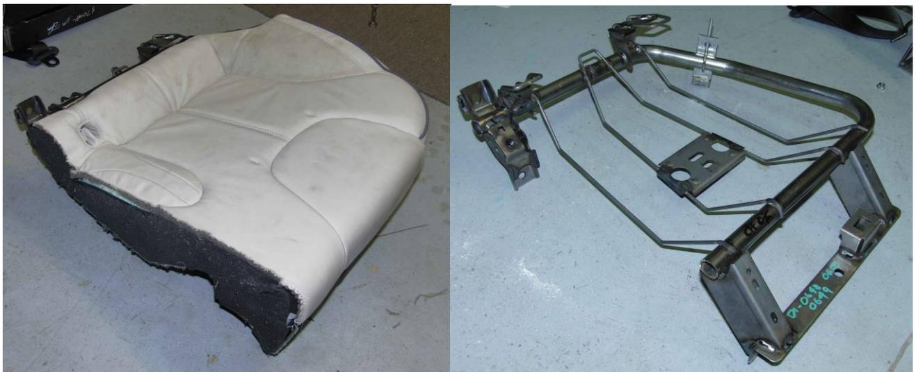
**Figure 5 The standard left passenger rear seat, showing the underlying structure.**
